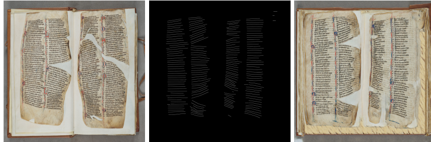
Fig. 4. Generation of damaged document. From Left to Right: Original document (real image), a generated mask, and an artificial image
